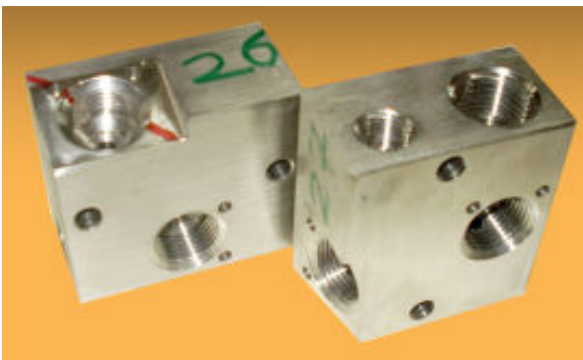
Sp4 - '2 valve' blocks manufactured by a steel industry are found to be contaminated
