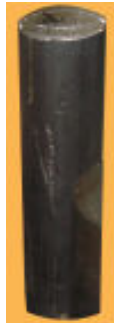
Sp7 - Steel rod sample from a steel industry found to have low level contamination
