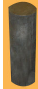
Sp5 - Steel rod sample from a steel industry found to have low level contamination
