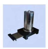
Detector material : Zns (Ag) Screen covered with Aluminized mylar foil
