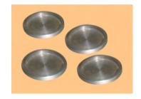
(B) ALPHA STANDARD SOURCE: Am241 alpha standard source can be supplied as an optional item. This is an electro deposited source on an SS planchet. Typical activity is in the range of 3000 to 5000 dpm.
