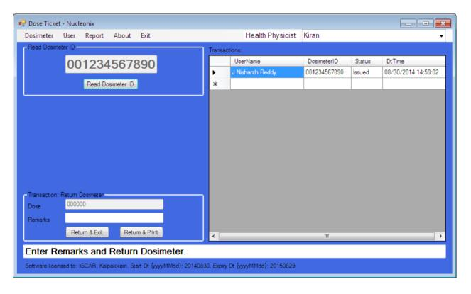
The Health Physicist can enter the remarks & click on either 'Return & Exit' button or in case Ticket printing is required, 'Return & Print' button can be clicked. The dosimeter's Dose value is nullified & it is automatically powered off upon Returning.
