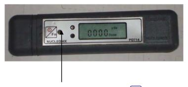
To switch OFF the equipment press the Fn key for 5 secs where the arrow is pointed to
