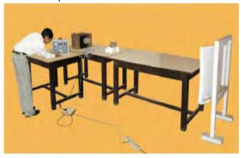
Gamma Survey instruments calibrator has Cs-137 source 161.5 mCi as on 05 Aug 2002. It is basically a gamma survey instruments calibrator procured from AEA Technologies UK/USA. Has NIST traceability accuracy within +/- 7%
