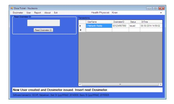
To return the dosimeter, insert the dosimeter in Docking station & click on 'Read Dosimeter ID' button. The screen looks like below:
