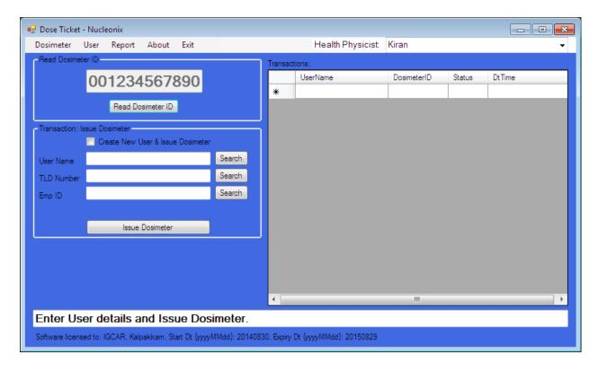
To assign the Dosimeter to a User, who is already in the database, type User Name / TLD Number / Emp ID and click on Search button. Then, click on 'Issue Dosimeter' button. The transaction is displayed in the Grid on right.
