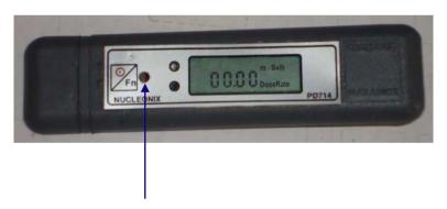
To check the measurement in DoseRate mode pressFn Key for 1 Sec.
