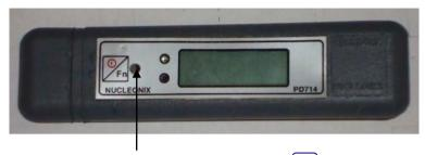
To switch ON the equipment press the Fn key for 1 sec where the arrow is pointed to
