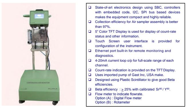
**Introduction :** Continuous Air Monitor, Type: NXG\_CAM\_BG manufactured by Nucleonix Systems, is a Plastic scintillator based continuous air monitoring system, designed using state-of-art electronics and is primarily used for, checking Beta activity present in the form of suspended particulate in air. It is very much essential to monitor the quality of air in & around Radiochemical plants, reprocessing plants in disaster scenario and other strategic locations.
