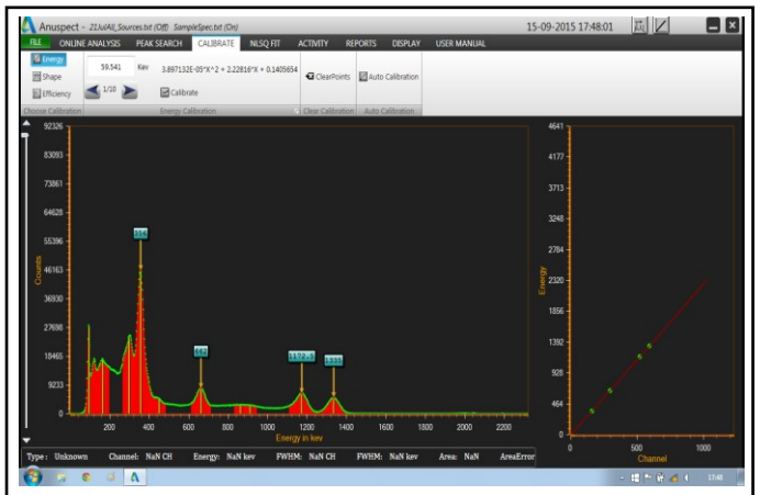
PHA spectrum, linearity chart by using NaI detector
